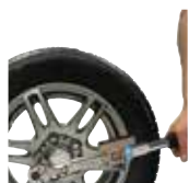
Completion of tightening process with Blue signal.
